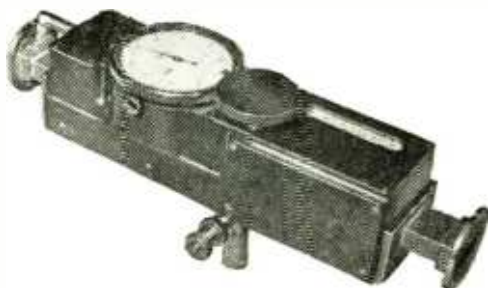
Standing-wave indicator for 3-cm band made by Elliott.
