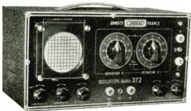
Servicing oscilloscope with 3-in. c.r. tube. (Centrad).
